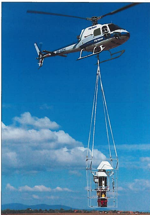
A Jet Ranger helicopter flew with the door removed from which poked a 4kW searchlight and below a 12kW generator.
